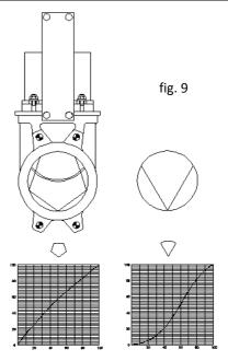
VERTICAL: MAXIMUM FLOW % HORIZONTAL: VALVE OPENING
